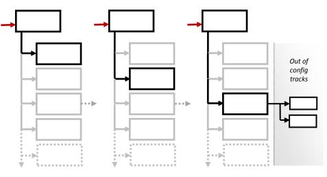
**Simple, efficient:** all tracks and routings that are part of the config<sup>2</sup> are muted except the active one! The main advantages of this solution are: immediate and seamless switching between configs (no disk access during switches: everything is already present in the project file + the tool obeys the REAPER preference > Audio > Track mute fade) as well as CPU savings (see 6).
