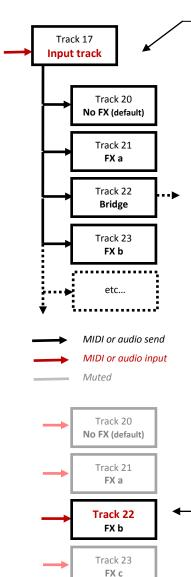
**Here is one example we will detail:** when it is started, REAPER automatically loads our project file<sup>1</sup> which contains an "input track" (i.e. an armed track without "Master/parent send") and all the FX we need on tracks 20 to 23 (or more). The MIDI or audio input is simply routed from the input track 17 to those tracks.
